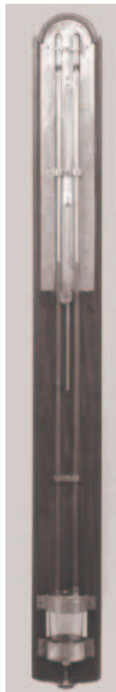
Photo 2. Fortin's mercury barometer (1788).
