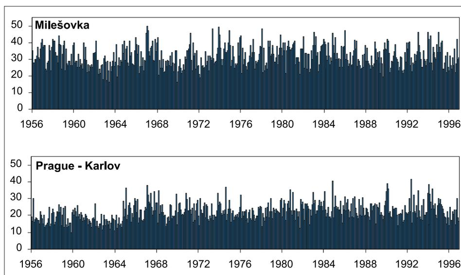
Fig. 1. Fluctuation of maximum monthly wind gusts ( $\text{m}\cdot\text{s}^{-1}$ ) at Mt. Milešovka and Prague-Karlov in 1956-1996. For Prague-Karlov the impairment of homogeneity after the exchange of the anemograph in October of 1964 is well perceptible.
